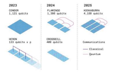
IBM expects to build quantum computers of increasing complexity over the next few years, starting with those that use the Condor processor or multiple Heron processors in parallel.
